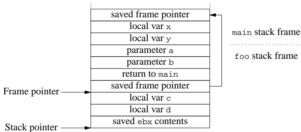
**Figure 3: Complete stack frame after entering called function**
