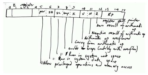
The SD bit determines the data space, and the SC bit determines the code space. The SG-relative addressing mode is an exception to this rule: it always addresses system data.
